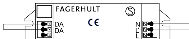
Setting DALI when used as a relay without a light source. If the RF unit is used, for example, for a whiteboard light, the DALI terminals shall not be short circuited.
