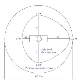
Example for light and motion detection area at height 1.7 m.
