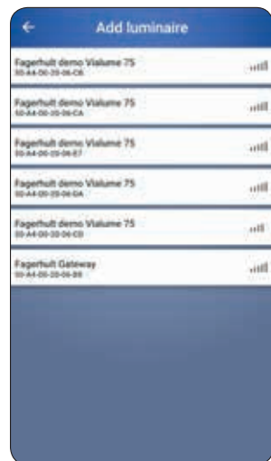
A list of luminaires in the vicinity will be displayed, sorted by signal strength. The top luminaire is likely the one you are at.
