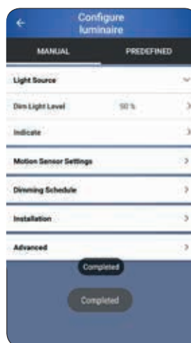
Completed is displayed when the luminaire has flashed.
