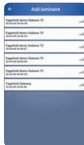
A list of nearby luminaires is displayed, arranged for signal strength. The top luminaire is probably the one you are at.
