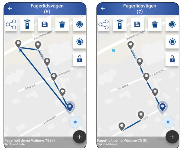
*Avoid creating links that form a continuous loop. Here, a link must be removed.*
