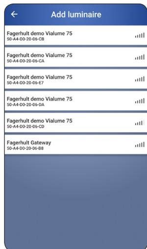
A list of luminaires in the vicinity will be displayed, sorted by signal strength. The top luminaire is likely the one you are at.
