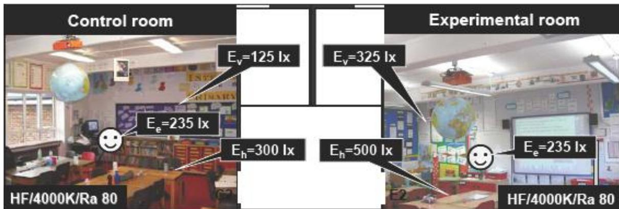
**Figure 2.** The figure shows the design of the control room vs. the experimental room and the horizontal and vertical illuminance as well as the type of fluorescent tubes.
