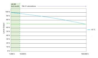
Data from the first 10.000 hours is used to extrapolate the expected time for i.e.  $L_{\rm yr}$ . The reached time is mainly depending on used LED and the temperature.
