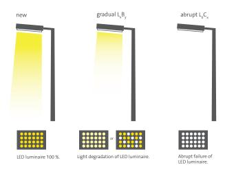
Explanation of the B- and C-value. Note that a failure of single LEDs on a multi LED-module is included in the B-value and not in the C-value.
