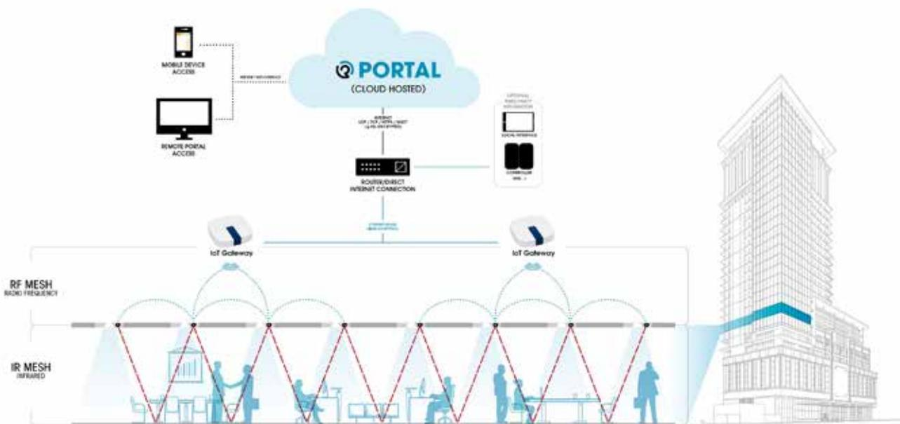
Each IoT-gateway must be in the communications range of at least one sensor node, i.e. within 5 metres in direct view. Each sensor node has the ability to connect to any gateway within the communications range, if there are multiple IoT-gateways close by. An IoT-gateway can in turn be connected to any DHCP network (Building specific) to forward and receive information from the e-Sense Organic Portal.
