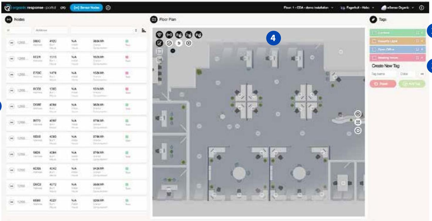
**1** Here you will find detailed information for each node. The information can be used during maintenance of the lighting installation. Click a row for one sensor, and the drawing will move to the location of the node.
