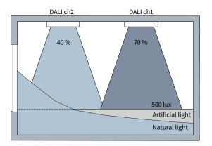
Example for a room with -30 % offset for channel 1. Channel 1 is brighter and light is further away from the window than channel 2. This will create an eve light level in the whole area.
