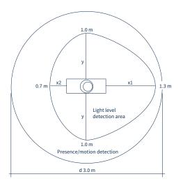
Example for light and motion detection area at height 1.7 m.
