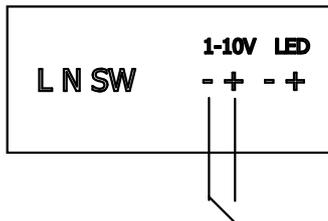
Short circuit 1-10v port for min 2 sec to reset the device
