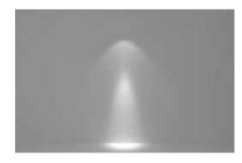
Spot is the narrow beam that will create great contrast. A narrow beam spotlight will be perceived as wider if it is a high ceiling height.
