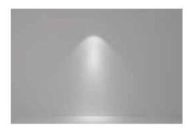
Luminaries with a medium beam angle are used to get a light that is less contrasting than a spot. Also, it does not give the sharp edges of a spot, but more a smoother distribution of light.
