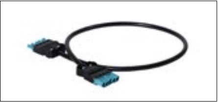
Connection cable, Wieland, 5-pin. 1-phase + dimming. 5 x 1.5 mm². L = 1.0 m, 2.0 m, 2.5 m, 3.0 m.
